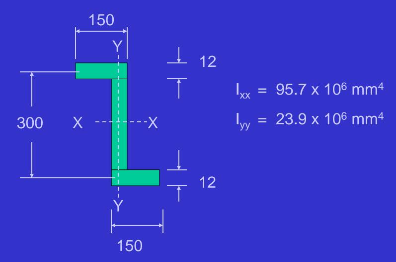
Now apply a hogging (positive) bending moment of  $M_x = 10 \text{ kN.m} = 10 \text{ x } 10^6 \text{ N.mm}$
