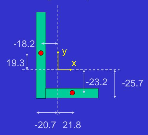
$$I_{xy} = (5 \times 90 \times -18.2 \times 19.3) + (5 \times 75 \times -23.2 \times 21.8)$$
