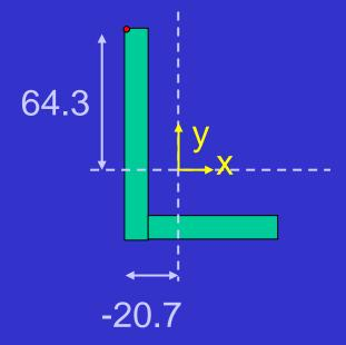
$$\sigma_{z} = \frac{\left(5 \times 10^{6} \times 5.04 \times 10^{5}\right)}{\left(5.04 \times 6.74 - 3.48^{2}\right) \times 10^{10}} \times 64.3$$
