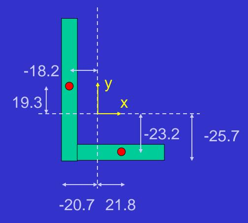
$$I_{xx} = \frac{5 \times 90^3}{12} + \left(5 \times 90 \times 19.3^2\right) + \frac{75 \times 5^3}{12} + \left(5 \times 75 \times -23.2^2\right)$$
