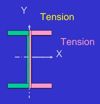
Define +ve M<sub>x</sub> as causing +ve tensile stresses when y is +ve
