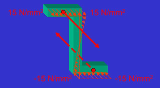
The forces in the flanges result in horizontal forces that are laterally out of alignment.
