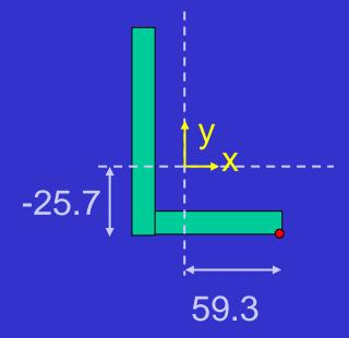
$$\sigma_z = \frac{2.52 \times 10^{12}}{2.20 \times 10^{11}} \times \left[ -25.7 \right] + \frac{1.73 \times 10^{12}}{2.20 \times 10^{11}} \times 59.3$$
