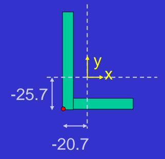
$$\sigma_z = \frac{2.52 \times 10^{12}}{2.20 \times 10^{11}} \times \left[ -25.7 \right] + \frac{1.73 \times 10^{12}}{2.20 \times 10^{11}} \times \left[ -20.7 \right]$$
